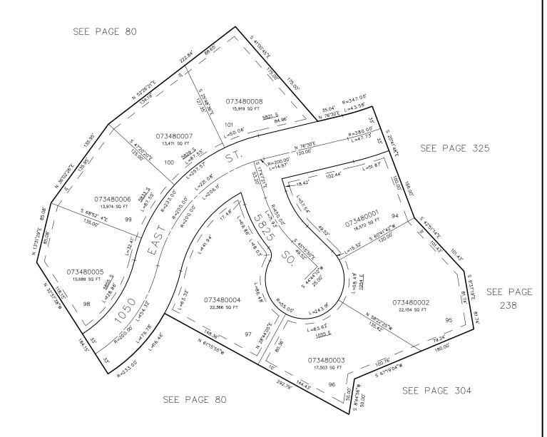
7' UTILITY & DRAINAGE EASEMENTS EACH SIDE OF PROPERTY LINE AS INDICATED BY DASHED LINES, EXCEPT AS OTHERWISE SHOWN.
